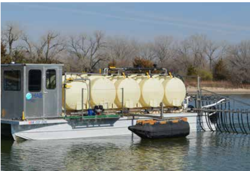
HAB (Cedar Lake's selected contractor) Alum Barge
